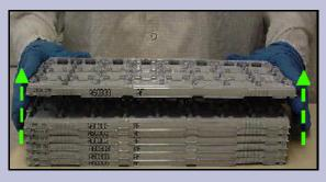
the product. In 2001, Intel engineers discovered a way to reduce by 58% the weight of the trays used to transport microprocessors by switching from injection-molded plastic to thermoformed plastic (PET). This innovation is yielding millions of dollars in annual savings and a reduction of over 1.5 million pounds of plastics material per year, with minimal up-front capital investment.
